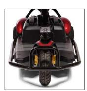
Front Bumper and Side Rails: Protect the scooter completely from impacts.
